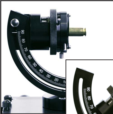
.40 cartridge casing held by the inside diameter
