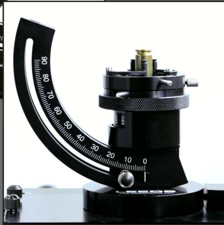
.40 cartridge casing held by the outside diameter
