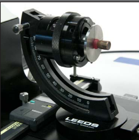
Bullet mounted with sticky wax to a mini platter
